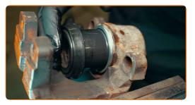
While continuing to push the piston carefully, insert it into the housing. Use a special brake caliper piston wind back tool
