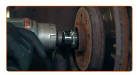
In most cases, when working with a steering knuckle, the CV axle should be disengaged
