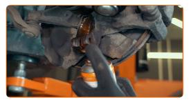
23 Install new fasteners
