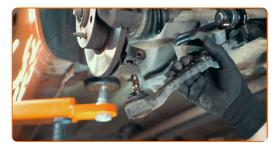
5 Detach any components obstructing access to the ball joint
