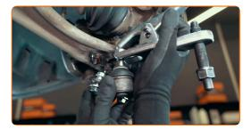
If using a puller is impossible due to lack of space, select another suitable tool
