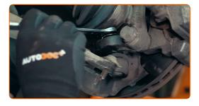
If the fastener is stuck, free it up before pressing the ball stud out of the steering knuckle
