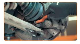
Traces of corrosion or dirt will prevent the new component from fitting properly
