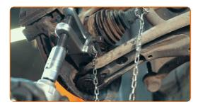
Rest the upper jaw of the tool against the ball stud and press the joint out of its mounting seat
