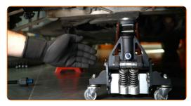
When using a jack, be sure to secure the car with jack stands and wheel chocks
