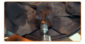
Treat the ball stud mounting seat with an anti-corrosion agent
