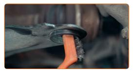
Carefully pry up the clip and remove the rubber element
