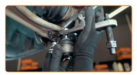
The ball joint can be removed with a ball joint puller. The lower jaw of the tool should be placed under a component, for example the steering knuckle, for support.
