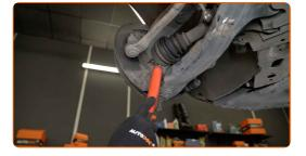
Remove the fasteners that connect the ball joint to the steering knuckle
