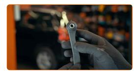
After tightening the link fasteners, treat them with an anti-corrosion agent
