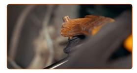
Install the fasteners one by one: tighten the first one just a little bit, then go on to the next one
