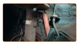
Coat the threaded parts of the link with an anti-corrosion agent
