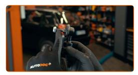
The fasteners of the drop links with rubber bushings should only be tightened after the car is lowered to the ground Otherwise, the bushings will rotate and get damaged, as well as the drop link itself.
