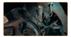
To prevent the stud from turning when tightening or unscrewing the fasteners, it should be secured by inserting an Allen key in a special slot
