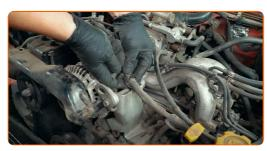
6 Unscrew the alternator fasteners.
