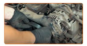
Disconnect the wiring after detaching its retainers.
