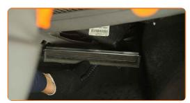
Screw in the fasteners of the cabin filter housing cover. Use a drive socket #7. Use a ratchet wrench.
