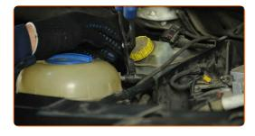
Detach the coolant tank hose. Use a flat screwdriver.
