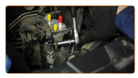
Connect the fuel lines to the new fuel filter.
