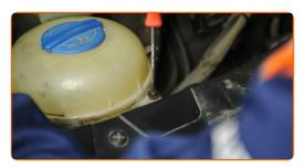
Attach the coolant tank hose.
