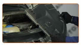
Detach the coolant expansion tank connector. Use a flat screwdriver.
