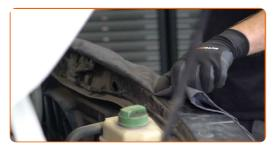
Remove the engine cover clips. Use a flat screwdriver.
