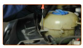
Remove the coolant reservoir.
