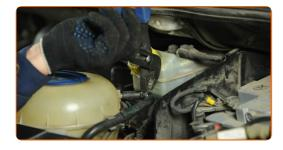
Attach the coolant expansion tank connector.
