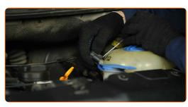
6 Loosen the coolant pipe clamp. Use clic-R collar pliers.
