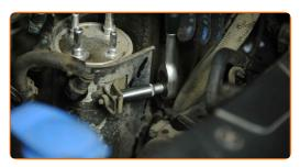
Remove the fuel filter. Use a flat screwdriver. Put the old filter cartridge in the container.
