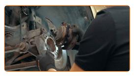
Remove the brake disc baffle plate.
