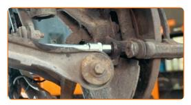
Remove the caliper bracket.
