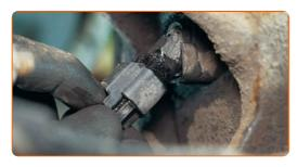
Clean the wheel hub fastener. Use a wire brush. Use WD-40 spray.
