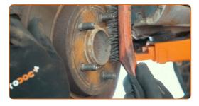
16 Unscrew the brake disc fastening.
