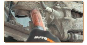
Release the parking brake cable. Use nippers. Use a crowbar.
