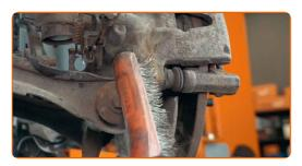
9 Unscrew the brake caliper fastening. Use a combination spanner #13.
