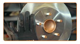
33 Screw in the brake disc fastener.
