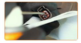
Attach the ABS sensor connector.
