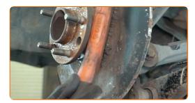
Unscrew the wheel hub bolts. Use Torx T50. Use a tap wrench.
