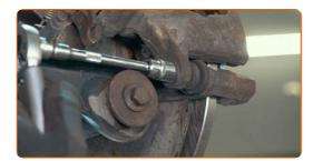
Install the parking brake cable into the brake caliper bracket. Use nippers. Use a crowbar.
