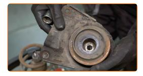
Release the coil spring.
