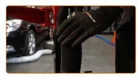
Install the spring on the shock absorber.
