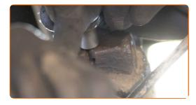
Detach the shock absorber from the rear knuckle.
