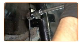
Treat the shock strut fasteners. Treat all joints of the stabiliser link. Treat the rear knuckle fasteners. Use copper grease.
