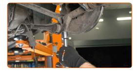
Tighten the fasteners connecting the control arm to the rear knuckle. Use a drive socket #15. Use a torque wrench. Tighten it to 103 Nm torque.
