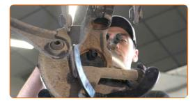
Clean the fasteners of the shock strut upper mount. Use a wire brush. Use WD-40 spray.
