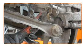
Release the parking brake cable. Use nippers. Use a crowbar.
