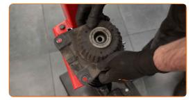
Tighten the shock strut piston rod nut. Use a drive socket #19. Use HEX No.H6. Use a torque wrench. Tighten it to 50 Nm torque.
