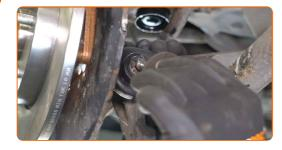
Screw in the fasteners connecting the control arm to the rear knuckle. Use a drive socket #15. Use a ratchet wrench.
