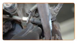
Clean the mounting seats of the stabiliser link. Use a wire brush. Use WD-40 spray.
