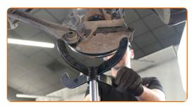
Release the fastener connecting the shock absorber to the rear knuckle. Use a special drive socket to remove the shock absorber. Use a ratchet wrench.
