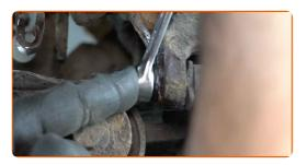
Remove the brake caliper. Use a crowbar.
