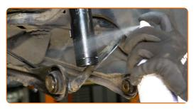
Attach the shock absorber to the rear knuckle.
