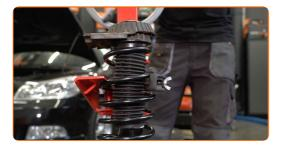
Remove the assembled shock strut.
