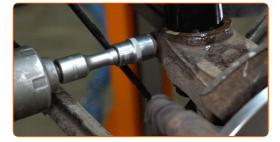
Attach the control arm. Install the fastening bolt.
