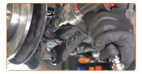
Attach the control arm. Install the fastening bolt.
