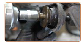
Remove the fastening bolt. Detach the control arm.
