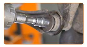
Attach the control arm. Install the fastening bolt.
