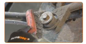
Unscrew the fastener connecting the control arm to the rear knuckle. Use a drive socket #15. Use a ratchet wrench.
