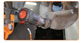
Remove the fastening bolt. Detach the control arm.
