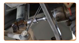
Remove the fastening bolt.
