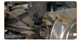
Screw in the fastener connecting the shock absorber to the rear knuckle. Use a drive socket #18. Use a ratchet wrench.
