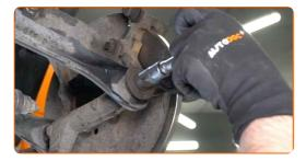
Tighten the fastener that connects the suspension strut to the rear knuckle. Use a drive socket #18. Use a torque wrench. Tighten it to 85 Nm torque.
