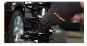
Clean the mounting seats of the shock strut. Use a wire brush. Use WD-40 spray.
