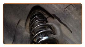
Secure the upper fasteners of the shock strut. Do not tighten it.
