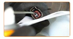
69 Attach the ABS sensor connector.
