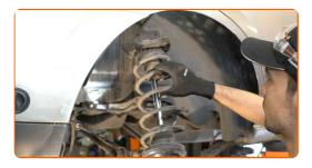
Set the shock absorber strut on the spring compressor tool.
