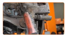
Unscrew the brake caliper fastening. Use a combination spanner #13.
