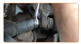
11 Remove the brake caliper. Use a crowbar.
