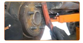
Unscrew the brake disc fastening.
