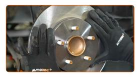
Screw in the brake disc fastener.
