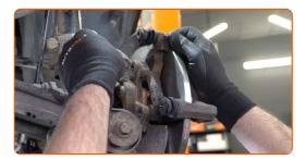
Tighten the brake caliper bracket. Use a drive socket #13. Use a torque wrench. Tighten it to 65 Nm torque.
