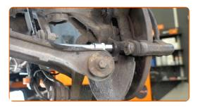
Remove the caliper bracket.
