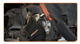
20 Install the brake disc.
