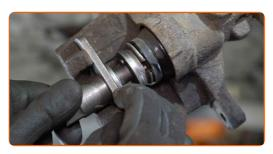
Install the brake caliper and fix it. Use a drive socket #13. Use a torque wrench. Tighten it to 30 Nm torque.
