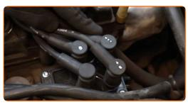
Disconnect the spark plug wires from the ignition coil. Disconnect the spark plug wires from the spark plugs.
