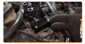
Treat the ignition coil connector with electronic spray.
