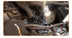
Tighten the ignition coil fastening. Use Torx T20. Use a torque wrench. Tighten it to 8 nm torque.
