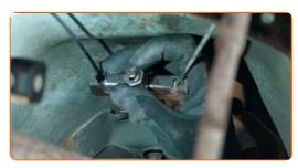
Release the parking brake cable. Use round-nose pliers.
