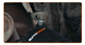
Remove the exhaust heat shield.
