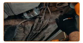
Detach the parking brake cable from the car body. Use a hammer. Use a crowbar.
