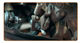
Adjust the parking brake cable tension. Use a drive socket #16. Use a ratchet wrench.
