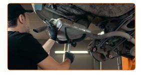
27 Attach the silencer to the bracket.
