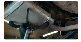
Unscrew the exhaust heat shield fasteners. Use a drive socket #10. Use a ratchet wrench.
