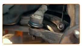
Screw on the fastening nut that connects the tie rod end to the steering knuckle. Use a drive socket #15. Use a ratchet wrench.
