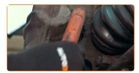
Unscrew the caliper bracket fastening. Use a drive socket #15. Use a ratchet wrench. Use a tap wrench.
