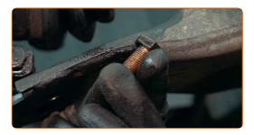
Clean the lower fastener connecting the suspension strut to the steering knuckle. Use a wire brush. Use WD-40 spray.
