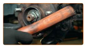
Treat the contacting surface. Use copper grease.
