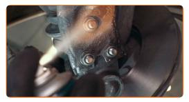
Treat the steering knuckle fasteners. Use copper grease.
