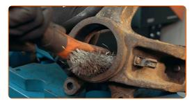
Pull the bearing inner race out of the wheel hub. Use a universal puller. Use a bush and bearing driver set.
