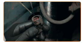
Attach the ABS sensor connector.
