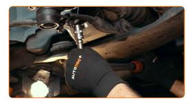
Tighten the lower fastening of the shock absorber. Use a drive socket #15. Use a torque wrench. Tighten it to 83 Nm torque.
