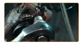
Remove the steering knuckle together with the hub. Use a hammer.
