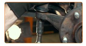
Tighten the fastening nut connecting the tie rod end to the steering knuckle. Use a drive socket #15. Use a torque wrench. Tighten it to 40 nm torque.
