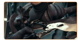
45 Attach the ball joint to the control arm.
