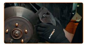
Tighten the brake caliper bracket. Use a drive socket #15. Use a torque wrench. Tighten it to 100 Nm torque.
