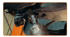
Tighten the fasteners connecting the ball joint to the control arm. Use a drive socket #17. Use a torque wrench. Tighten it to 44 Nm torque.
