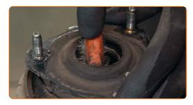
Unscrew the strut piston rod nut. Use a drive socket #19. Use HEX No.H6. Use a ratchet wrench.
