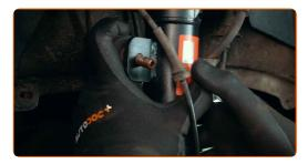
Tighten the stabiliser link fastener. Use a drive socket #17. Use a ratchet wrench.
