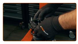
Tighten the shock strut piston rod nut. Use a drive socket #19. Use HEX No.H6. Use a torque wrench. Tighten it to 55 Nm torque.
