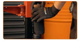
Install the spring on the shock absorber.
