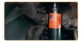
74 Treat the shock strut fasteners. Treat the steering knuckle fasteners. Use copper grease.
