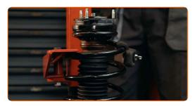
Remove the assembled shock strut.
