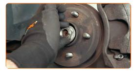
Screw the nut of the drive shaft. Use a drive socket #32. Use a ratchet wrench.
