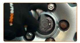
6 Loosen the fastener of the driveshaft. Use a drive socket #32. Use a tap wrench.
