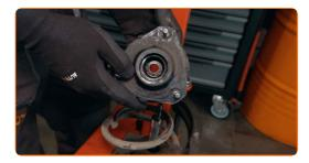
Release the coil spring.
