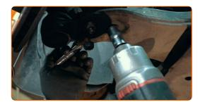
Tighten the fasteners connecting the ball joint to the control arm. Use a drive socket #17. Use a torque wrench. Tighten it to 48 Nm torque.
