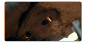
Screw in the fastener connecting the ball joint to the control arm. Use a combination spanner #17. Use a drive socket #17. Use a ratchet wrench.
