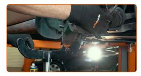
Release the lower fastener connecting the shock strut to the steering knuckle. Use a special drive socket to remove the shock absorber. Use a ratchet wrench.
