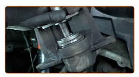
Install the brake caliper and fix it. Use a combination spanner #19. Use a drive socket #13. Use a torque wrench. Tighten it to 30 Nm torque.
