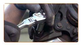
10 Remove the brake caliper.
