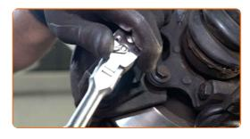
10 Remove the brake caliper.
