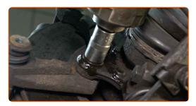
14 Remove the caliper bracket.
