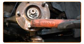
17 Install the brake disc.
