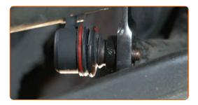
Tighten the fastener connecting the stabilizer link to the shock strut. Use a combination spanner #17. Use a drive socket #17. Use a torque wrench. Tighten it to 48 Nm torque.
