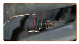
Tighten the stabiliser link fastener. Use a combination spanner #17. Use a drive socket #17. Use a ratchet wrench.
