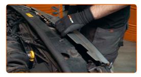
Screw in the fastener of the radiator grille.
