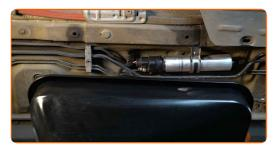
Remove the snap ring of the fuel pressure regulator retainer clip. Use a flat screwdriver.
