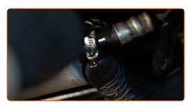
Clean the fuel filter mounting bracket. Use all-purpose cleaning spray.
