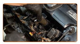
Plug in the ignition coil connector.
