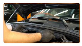
Reinstall the cabin filter housing cover. Make sure you hear a click indicating that it is locked in place.
