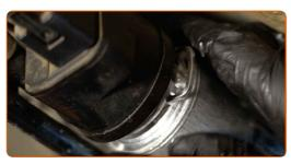
Screw in the fuel filter mounting bracket. Use a drive socket #10. Use a ratchet wrench.
