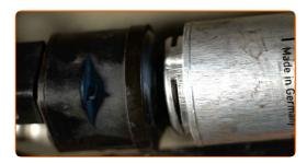
Install the snap ring of the fuel pressure regulator's retainer clip.
