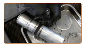
9 Remove the fuel filter fastening bracket.
