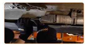
Detach the fuel pressure regulator from the fuel filter. Use a crowbar.
