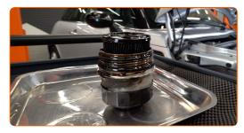
Cover the oil filter housing with a microfibre towel to prevent dirt and foreign objects from getting into the system.
