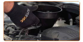
Pour oil into the engine through the filler. Required amount of oil: 4.8 l.
