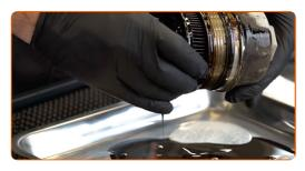
Install a new O-ring to its mounting seat on the filter cover. 14
