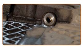
Screw in the new drainage plug and tighten it. Use a drive socket #13. Use a torque wrench. Tighten it to 25 Nm 17 torque.
