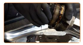
Remove the oil filter cover O-ring. 13
