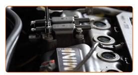
Install the spark plug wire connectors into the spark plug wells. Connect the spark plug wires to the ignition coil.
