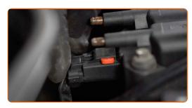
Unscrew the ignition coil bracket. Use a drive socket #10. Use a ratchet wrench.
