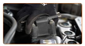
Treat the ignition coil tips. Use high-temperature grease. Use a flat screwdriver.
