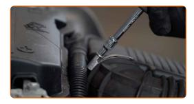
Undo the fastening screws of the air filter cover. Use a drive socket #8. Use a ratchet wrench.
