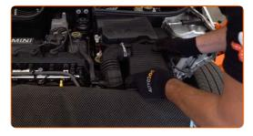
Attach the air intake hose to the air filter housing. Tighten the fuel filter pipe clamp. Use a drive socket #6.
