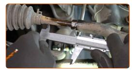
Loosen the lock nut securing the tie rod end to the tie rod. Use a combination spanner #17. Use a combination spanner #19.
