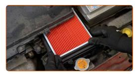
Install the air filter housing.
