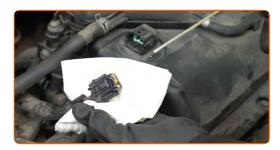
Attach the connectors to the engine cover. Use a flat screwdriver.
