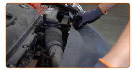
Disconnect the fastener of the air intake hose. Use a clip removal tool.
