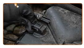
Insert the filter cartridge into the filter housing.
