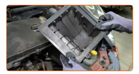
Detach the connectors from the engine cover. Use a flat screwdriver.
