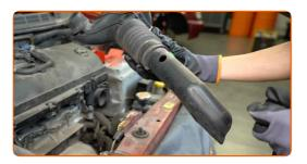
Release the air filter housing retainers.
