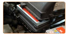
Lock the air filter housing retainers.
