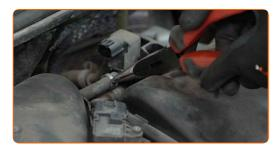
Unscrew the fasteners of the upper engine cover. Use a drive socket #10. Use a ratchet wrench.
