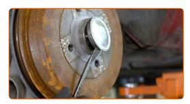
Unscrew the wheel hub fastener. Use a drive socket #30. Use a tap wrench.
