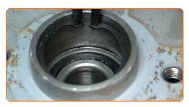
Press out the wheel hub bearing. Use a bush and bearing driver set.
