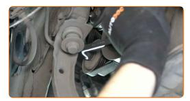
Loosen the serpentine belt. Use a drive socket #12. Use a ratchet wrench.
