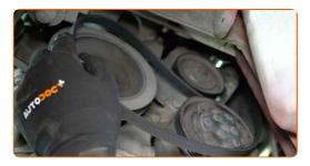
Loosen the tensioner pulley fastener. Use a combination spanner #14.
