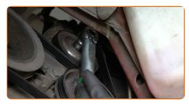
Rotate the crankshaft several times to make sure the new V-ribbed belts are working properly. Use a drive socket #27. Use a ratchet wrench.
