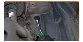
Loosen the tensioner pulley fastener. Use a combination spanner #14.
