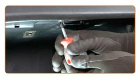
Remove the glove box cover retainers.
