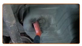
Unscrew the drain plug. Use a drive socket #14. Use a ratchet wrench.
