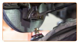
12 Unscrew the rear fastener of the control arm. Use a combination spanner #18. Use a drive socket #18. Use a ratchet wrench.
