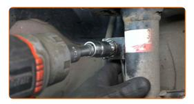
Disconnect the sway bar link from the suspension strut.
