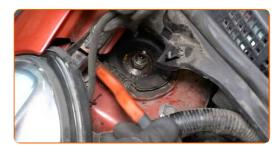
Loosen the upper fasteners of the suspension strut. Use a drive socket #13. Use a ratchet wrench.
