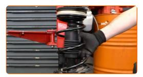
Clean the mounting seats of the shock strut. Use a wire brush. Use all-purpose cleaning spray.
