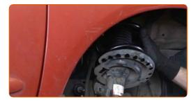
Secure the upper fasteners of the shock strut.
