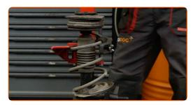
Clean the strut piston rod. Use a wire brush. Use WD-40 spray.
