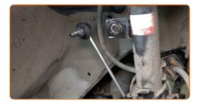
Disconnect the ABS sensor wiring.
