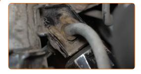
Connect the ABS sensor wiring.
