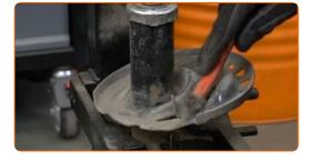
Install the dust boot and bump stop on the shock absorber.
