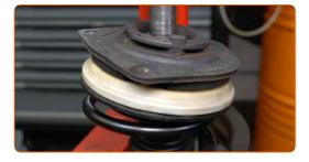
Tighten the nut of the suspension strut piston rod. Use a 18-mm strut nut socket. Use HEX No.H6. Use a torque wrench. Tighten it to 68 Nm torque.
