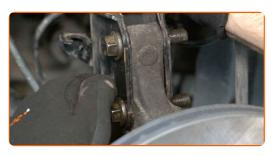
Fasten the brake hose on the strut.
