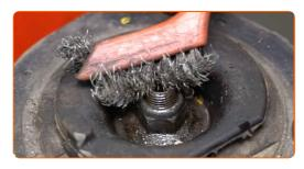
Unscrew the strut piston rod nut. Use a 18-mm strut nut socket. Use HEX No.H6. Use a ratchet wrench.
