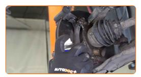
Unscrew the brake caliper bracket fasteners. Use a drive socket #17. Use a ratchet wrench.
