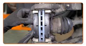
Install the brake caliper and fasten it.
