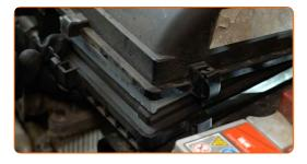
Lock the air filter housing retainers.
