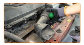
Release the air filter housing retainers.
