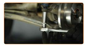
Tighten the tie rod end locknut. Use a combination spanner #19. Use a torque wrench. Tighten it to 65 nm torque.
