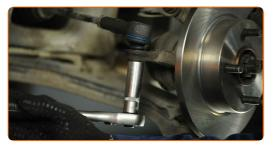
Treat the fastener connecting the tie rod end to the steering knuckle. Treat the shock strut fasteners. Treat the fasteners of the ball joint. Use copper grease.
