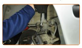
Fasten the brake hose on the strut.
