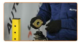
Tighten the upper fastener of the shock absorber strut mount. Use a combination spanner #14. Use an adjustable wrench. Use a torque wrench. Tighten it to 40 Nm torque.
