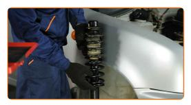
Secure the upper fasteners of the shock strut (3 pieces).
