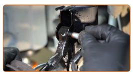
Tighten the lower fasteners connecting the shock strut to the steering knuckle. Use a combination spanner #17. Use a drive socket #17. Use a torque wrench. Tighten it to 115 Nm torque.
