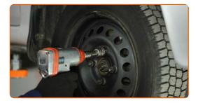
Lower the car and working in a cross order, tighten the wheel bolts. Use wheel impact socket #19. Use a torque wrench. Tighten it to 110 Nm torque.
