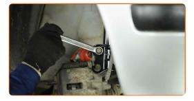
Fasten the brake hose on the strut.
