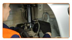
Treat the shock strut fasteners. Use copper grease.
