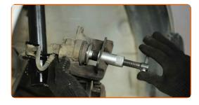
30.1 Install the brake caliper and fix it.
