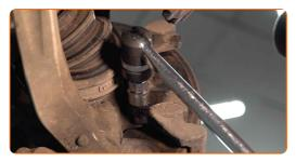
Remove the caliper bracket.
