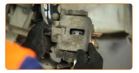
30.2 Use a drive socket #12. Use a torque wrench. Tighten it to 30 Nm torque.
