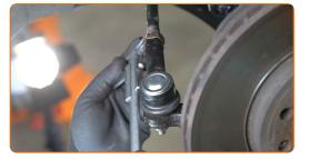
18 Tighten the tie rod end locknut. Use a combination spanner #21 (2 pieces). Use a torque wrench. Tighten it to 55 nm torque.
