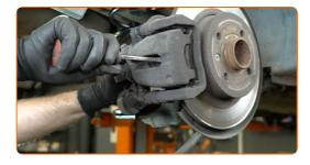
11 Remove the brake caliper.
