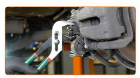
Unscrew the brake caliper fastening. Use a combination spanner #13. Use a combination spanner #17.
