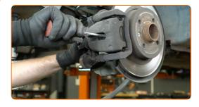
11 Remove the brake caliper.
