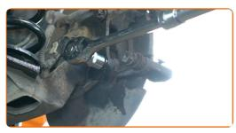
Remove the caliper bracket.
