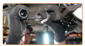
Install the brake caliper and fix it. Use a combination spanner #17. Use a drive socket #13. Use a torque wrench. Tighten it to 25 nm torque.
