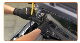
Unscrew the fasteners of the windscreen wiper scuttle tray. Use a drive socket #8. Use a ratchet wrench.
