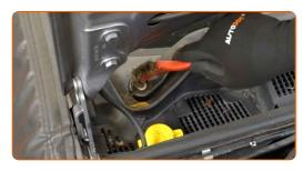
Unscrew the fasteners of the windscreen wiper arms. Use a drive socket #13. Use a ratchet wrench.
