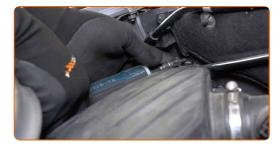
10 Release the engine bulkhead panel clips.
