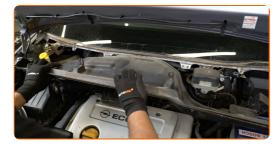
Screw in the fasteners of the windscreen wiper scuttle tray. Use a drive socket #8. Use a ratchet wrench.
