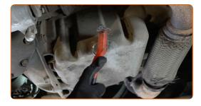
Unscrew the drain plug. Use Torx T40. Use a ratchet wrench.
