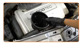
Pour oil into the engine through the filler. Required amount of oil: 3.5 l.
