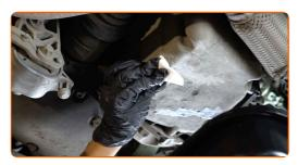
Screw in the new drainage plug and tighten it. Use Torx T40. Use a torque wrench. Tighten it to 24 Nm torque.
