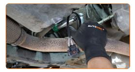
Treat the oxygen sensor connector. Use dielectric grease.
