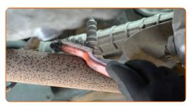
6 Unscrew the oxygen sensor fastener. Use a flare nut spanner #22.
