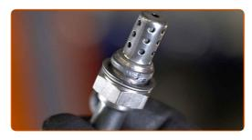
10 Install the new oxygen sensor.
