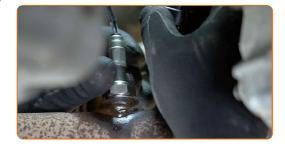
Tighten the oxygen sensor fastener. Use a drive socket #22. Use a torque wrench. Tighten it to 31 Nm torque.
