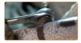
7 Remove the oxygen sensor.
