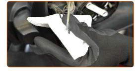
Attach the mirror heating connectors.
