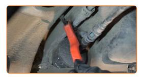
Disconnect the fuel supply lines from the fuel filter. Use fuel line pliers. Use a crowbar.
