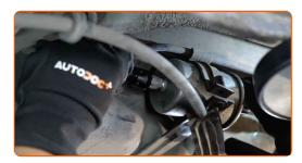
Screw in the fuel filter mounting bracket. Use a Phillips screwdriver.
